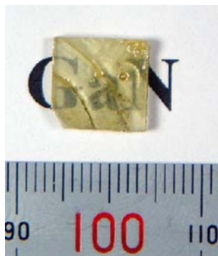
Fig. 1 Image of a 0.2 mm thick ammonothermal GaN crystal grown on (0001)HVPE GaN substrate
